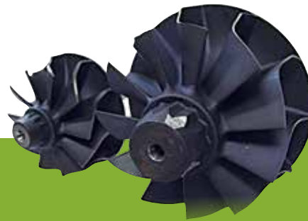
EFR 58mm and 80mm Gamma-Ti turbine wheels
