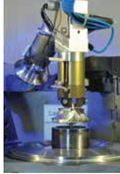
Forged-milled compressor wheel production
