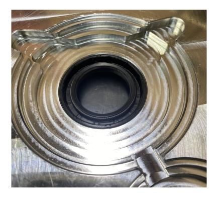
The input shaft seal then gets pressed into the plate as seen below
