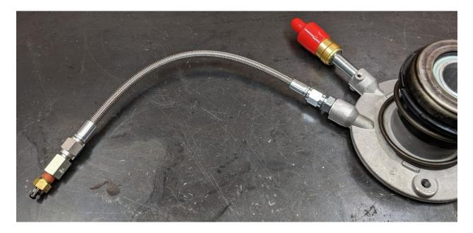
Once you have converted the TOB to -4 fittings, mount it to the plate with the 2 small screws, and run the lines through the B-Hole<sup>™</sup>. The transmission side of installation is now complete!
