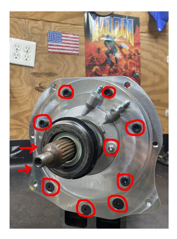
Note the 6 socket head screws at the top and the 3 countersunk bolts at the bottom. Mount the TOB with the two retaining screws to the plate, and make sure the lines are facing up. Multiple options are included depending on what is the easiest way to mount for your setup, including RHD options.
