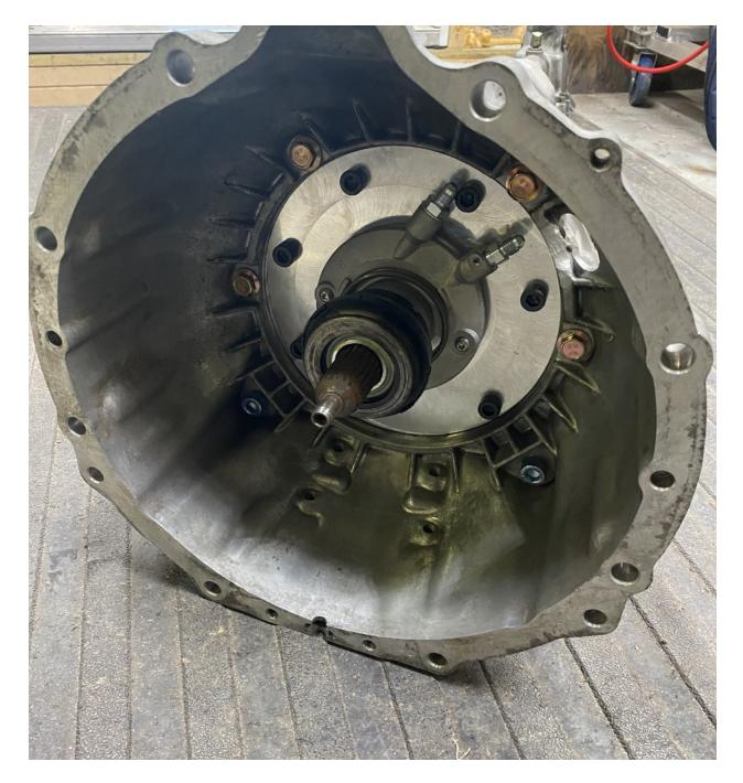
Now you will run your lines through the B-Hole<sup>™</sup>, install your flywheel to your engine, install the clutch to the flywheel, and bolt the transmission to the engine as if it came that way from the factory! Don't forget to use thread *sealant* on the flywheel to crankshaft bolts, and grease the input shaft splines just enough for the clutch disc to easily glide on
