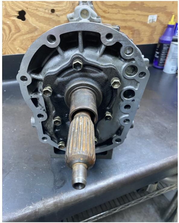
Now on to the transmission itself. Remove the bellhousing that is attached to the transmission. The next few pictures will be of a W55/W58 transmission, but the process is the same for the R series as well. The bolt pattern is completely different on the R series transmission, so they are not interchangeable. You will also need to remove the front bearing retainer as seen in the next picture. This is not reused, and is replaced by the XAT adapter plate.
