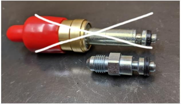
The side with the rubber seal goes in the TOB. The -4 side is for your hydraulic clutch line that goes up to your master cylinder.
