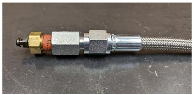
This setup is designed to be flexible and bleed any air in the hydraulic system from a convenient, serviceable point with the transmission and clutch fully installed.
