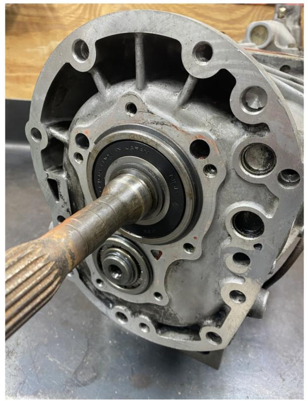
Make sure the mating surface of the plate/bearing retainer is completely flat and clean You can see where the old FIPG was that we scraped off.
