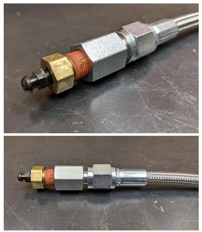
This setup is designed to be flexible and bleed any air in the hydraulic system from a convenient, serviceable point with the transmission and clutch fully installed.
