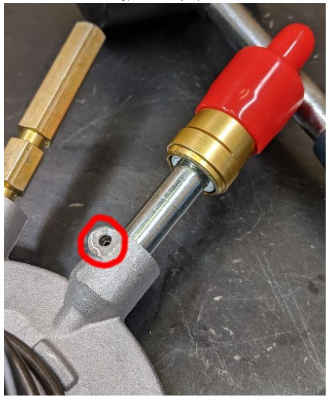
You will need to drive out the retaining pin for the GM style input into the TOB.
