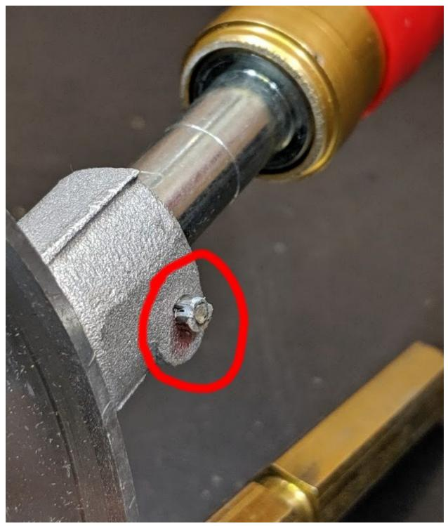
This GM fitting gets replaced with the silver -4 to quick disconnect fitting, and you will **reuse the retaining pin** that was driven out to hold this new fitting in place. The actual GM style fitting becomes a bonus part; it is superfluous.
