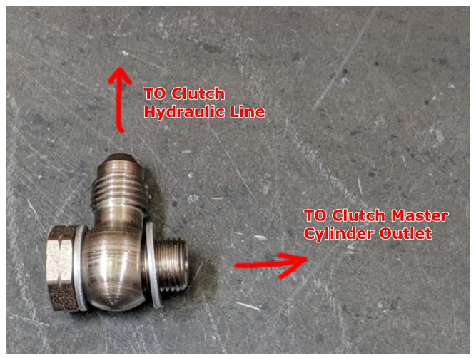
We offer options for these lines, however, we do not have a guaranteed-to-fit clutch line for *every* chassis on hand. **Please contact us with the length you need, and we can get a line made for you. This line is typically less than \$65 for a full length, stainless braided -4 line.** Once this has been done, the feed side will now be converted to -4 AN.
