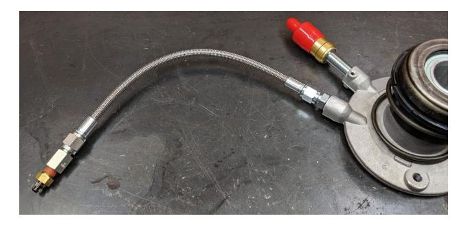
Once you have converted the TOB to -4 fittings, mount it to the plate with the 2 small screws, and run the lines through the B-Hole<sup>™</sup>. The transmission side of installation is now complete!
