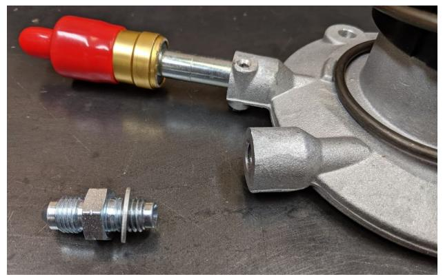
Then, attach the short (usually 10 inch) stainless braided bleed line to this end. You will install the ½ NPT to -4 Aeroquip adapter fitting on the small bleeder screw (this is bronze colored, has the black top and the red thread locker compound male side), which goes on the other end of the 10" bleeder line, and through the bellhousing for ease of access.
