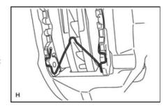
(g) Install the front disc brake anti-rattle spring to the disc brake caliper.
