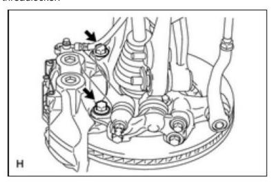
Step 10. Remove the 14mm banjo bolt from the stock caliper and install on the LS460 caliper. This spec is **29 ft lbs**. Again, we strongly recommend going with stainless braided lines while you're at it, which will also include new installation hardware.
