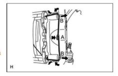
Note the head of the pin is facing in towards the vehicle. When you slide in the pin, we typically recommend using anti-seize on it, and also make sure the pin holes are pointing straight up during installation.
