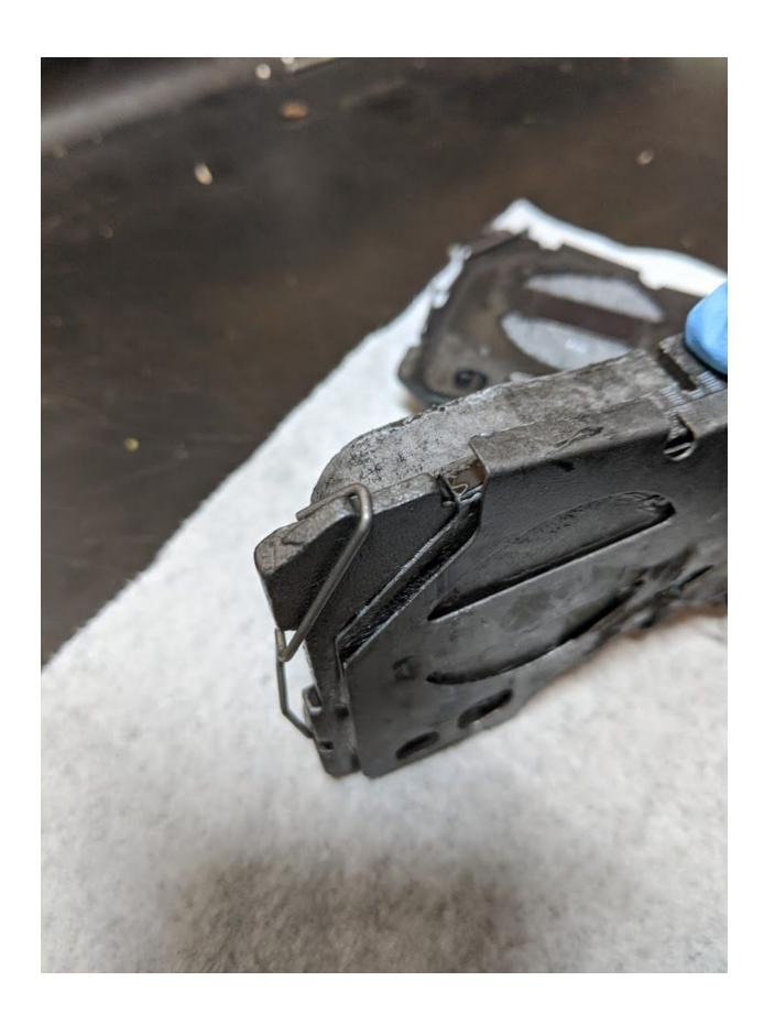
Make sure each of the caliper pistons have been fully retracted. If they are not, you will have quite a bit of trouble installing the thicc new brake pads. Slide the new pads in from the top of the caliper after it is installed.
