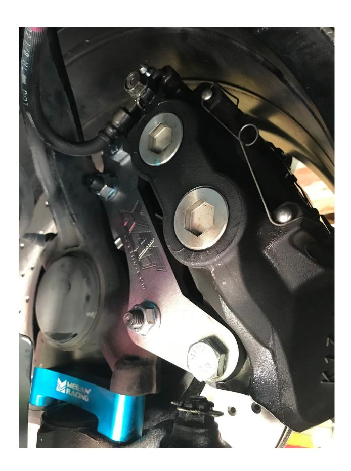
Step 12. After proper bleeding procedure of your brake system, you can reinstall your wheels and lower the vehicle back down. Torque wheel lugs to OEM spec after vehicle is on ground, usually 80-100 ft lbs.
