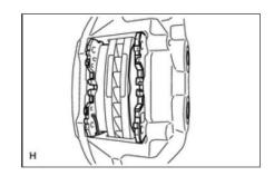
(f) Install the front disc brake anti-rattle spring between the 2 pads.
