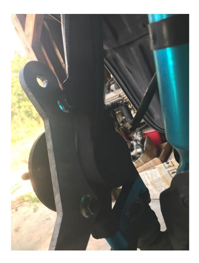
Step 8. Install new 14" vented rotor. This is a front 2008-2012 IS-F off the shelf rotor, though we typically supply StopTech/Centric since they're an OEM manufacturer, and we've yet to have any issues with them.
